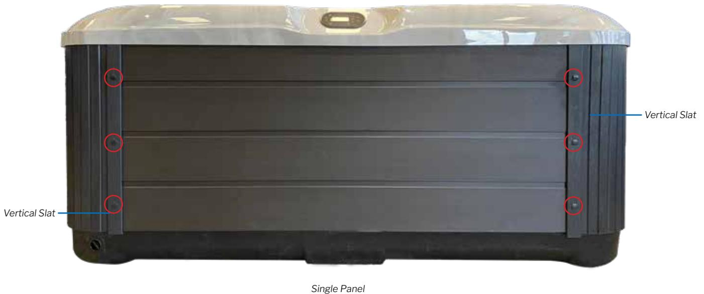
Each side of the spa pool consists a single cabinet panel. Holding each panel onto the frame of the spa pool are two vertical slats at each end with 3 screws per piece, with screw caps over each screw (circled on the diagram above).
