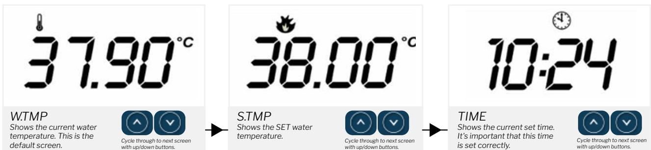
It's recommended to leave the display on WTMP to see a clear difference between your set temperature and your current water temperature.
