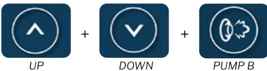
**NOTE:** 'Pump A' is the only visible jet button on the touch panel. 'Pump B' is a "ghost button" which is located to the right of Pump A which is activated by pressing down on the blank spot.
